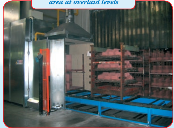
Example of pallets unloading area at overlaid levels
