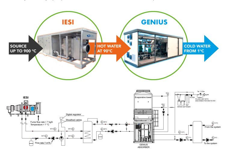
The diagram is to be considered indicative and not binding, as each IESI system is custom-built, according to the actual plant requirements and application needs of the customer.
